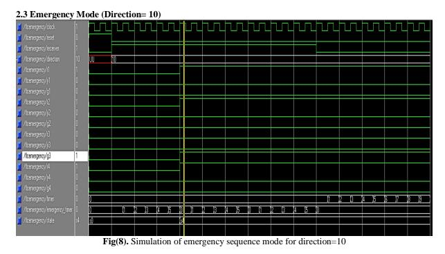
Figure shows the simulation of emergency sequence mode for west direction. As the receiver detected an ambulance and direction is 10 hence the system is in the state S4 that is G3 is ON. Similar to the previous stages, the emergency timer played its role, after receiver goes low the system is back in the normal sequence mode.
