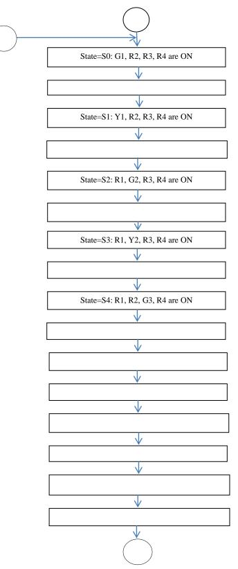
Fig(3). Flowchart for normal sequence mode.
