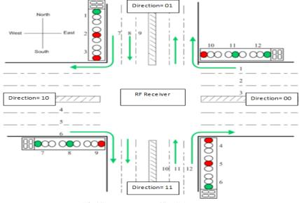
Fig(1). Four way traffic light system
