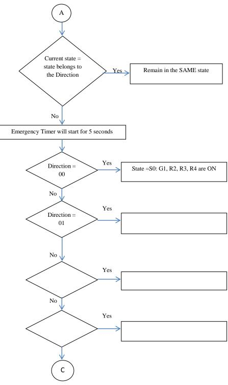
Fig(4). Flowchart for emergency sequence mode.
